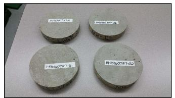
Photo 3. Specimens of the light weight structural concrete and regular weight concrete utilized to make both the slabs and specimens in Photos 1 and 2. These specimens were utilized for ASTM E96 vapor transmission testing. SRI Photo
