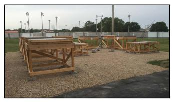
Photo 2. An overall view of the exterior slabs and smaller sample pans, exposed to the full weather, at SRI Consultants facility Wisconsin. SRI Photo
